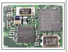
The configuration interface and transmit / receive FIFOs of the MXR-EM20 are accessed via a SPI interface.
