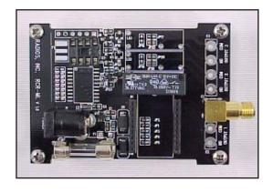
receiver allows a variety of antenna options for an SMA connector. Power is supplied through either a convenient wall-mount adapter or pig-tail connectors with an on-board fuse. Mounting can be done via the four 1/8" diameter mounting holes in each corner of the board. The RCR-ML operates at low power consumption, generates low harmonic emissions and is a highly reliable wireless link.
